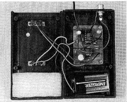
FIG. 4—THE INSIDE OF THE COMPLETED UNIT. You can use the same case (see the Parts List) or any other that will accept the board and a 9-volt battery.
