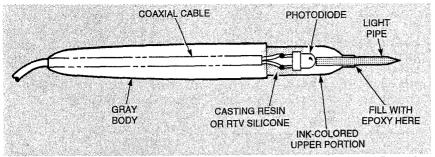
FIG. 5—CUTAWAY VIEW OF THE PROBE. The probe case was made from a fine-point feit-tip marker pen.
