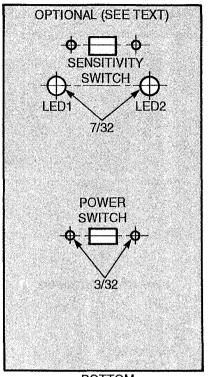
BOTTOM FIG. 3—DRILL GUIDE. S2 is optional, so don't drill holes for mounting it if you're not using it.
